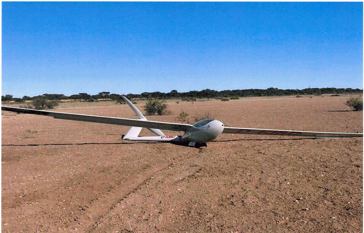
Photo 3 Photo depicting the ground scars by the aircraft and dry pan used for landing.
