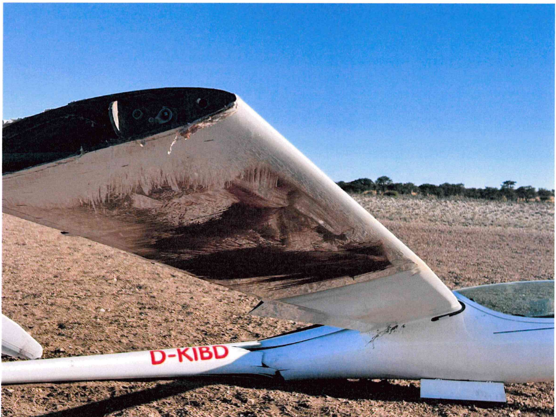
Photo 5 Photo depicting the aircrafts damage to right wing.
