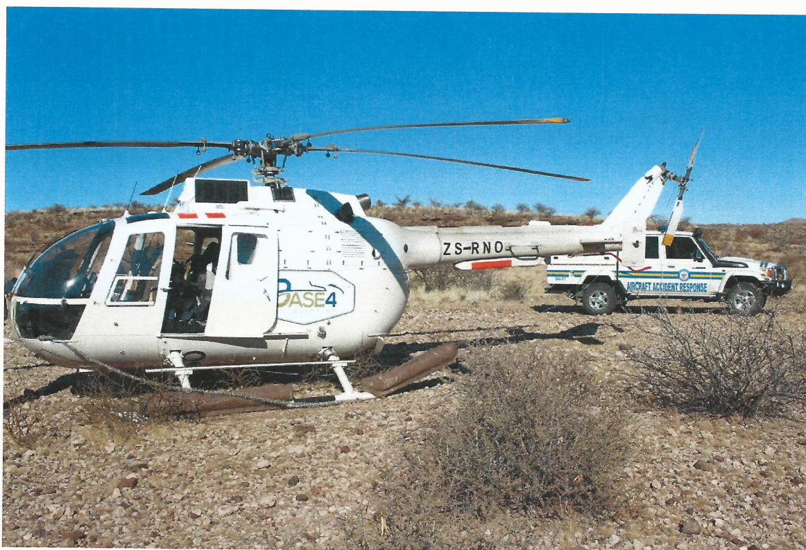
Figure 1. A photo showing where the helicopter landed and the electrical power line entangled around it.
