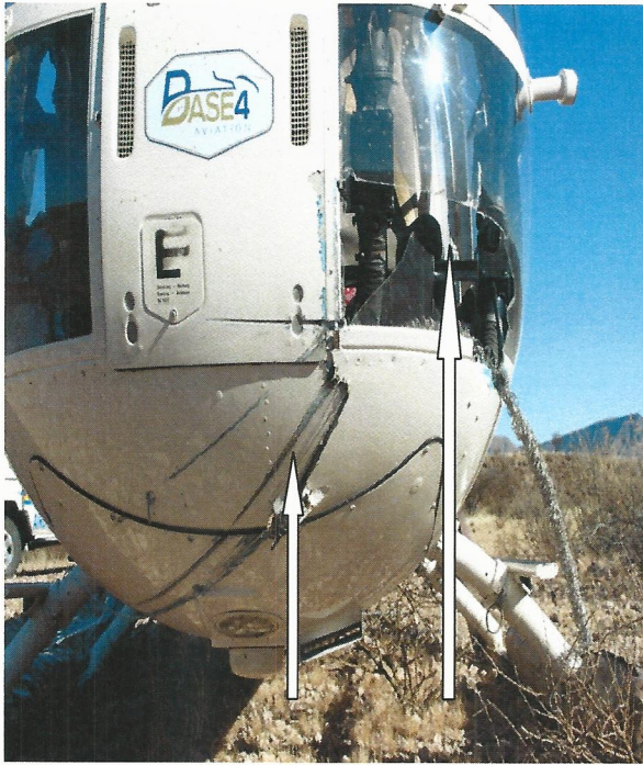
FIGURE 1: Nose section and windscreen damaged by the electrical cable.
