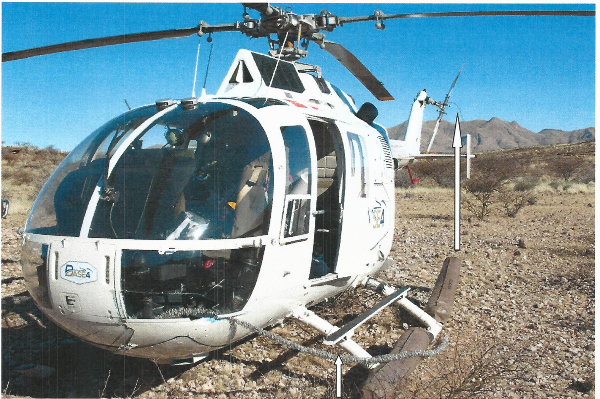
FIGURE 3: Photo showing the entangled cable.
