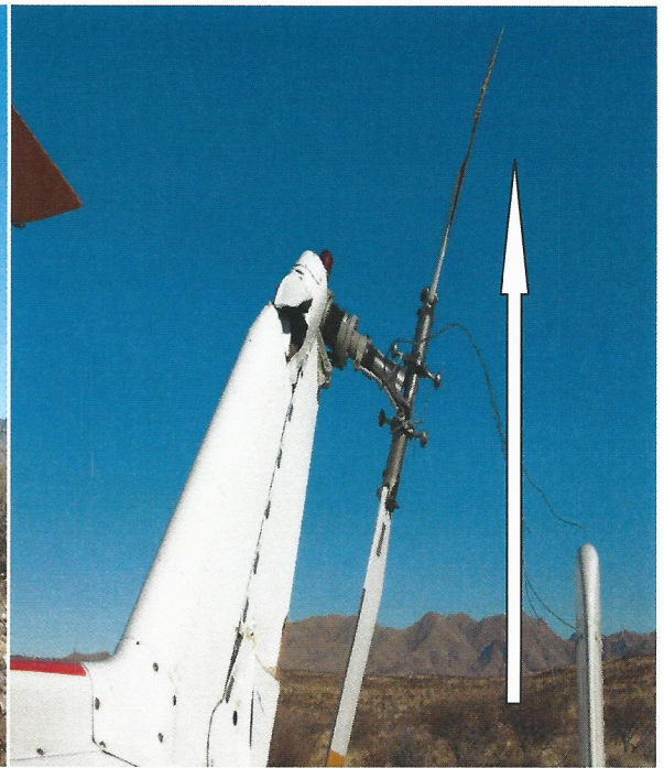
FIGURE 2: The tail rotor section and blades damaged
