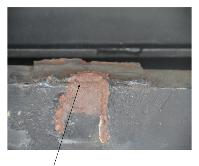
A place to where one of the missing central stow position support assembly use to be attached.
