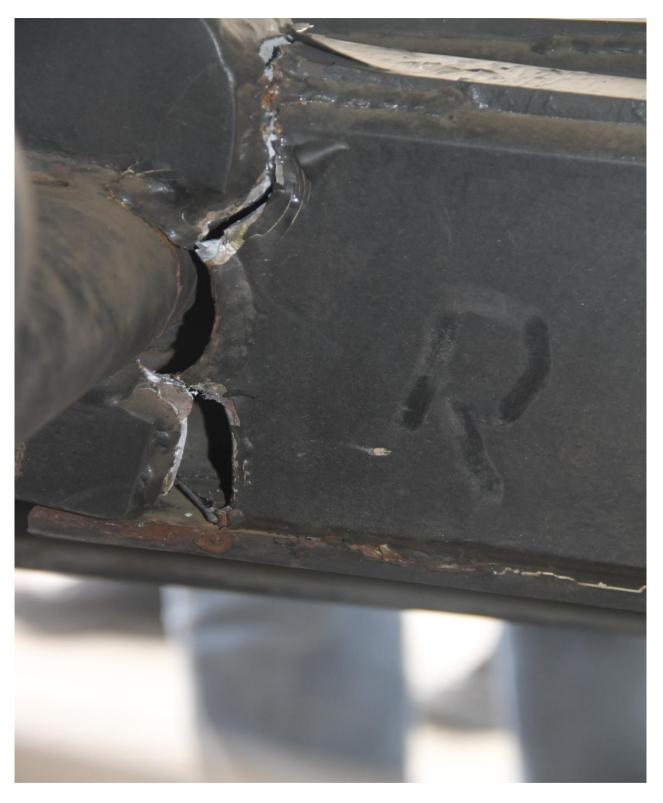
Appendix 4: A closer view of the crack on the left hand (L/H) side to where the lifting scissor is attached to the torque shaft.
