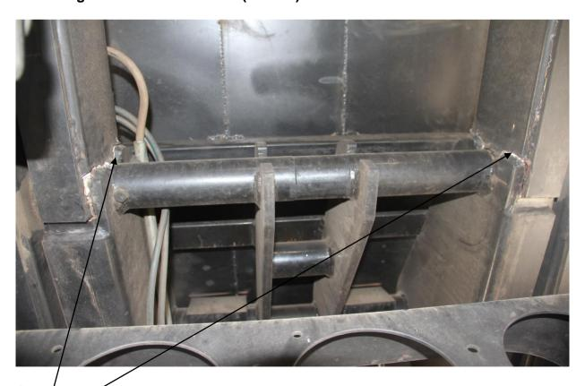
Cracks on both sides of the torque shaft.
