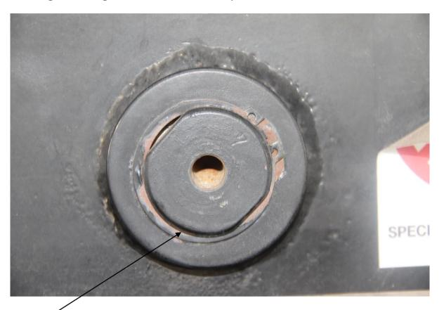
A bushing on the left side of the torque shaft that held the shaft in its position. The dryness and corrosion gives a sign that the equipment has not been lubricated for a long time.
