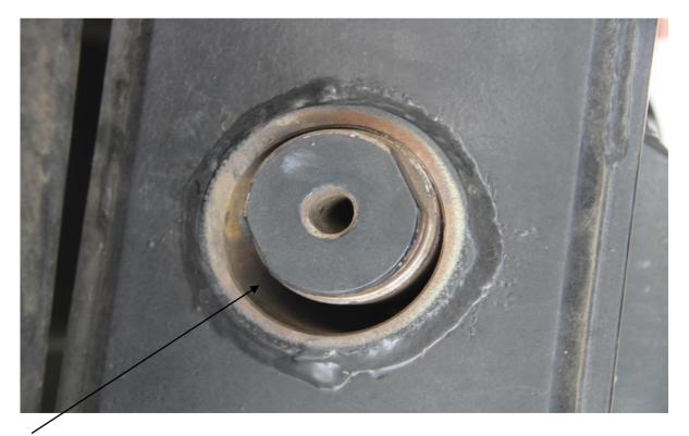
An opening space displaying a missing bushing on the right side of the torque shaft.
