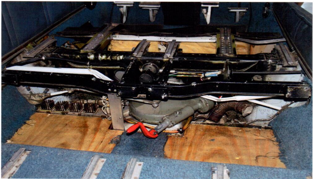
Figure 5: Depicting the landing gear Manual (emergency) extension system.
