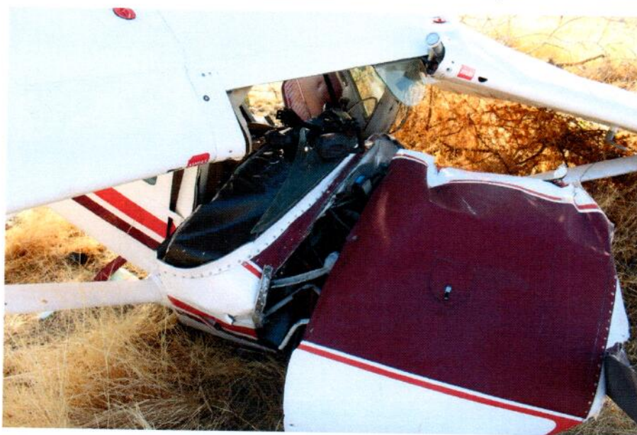
Image 5: Downward forces crushed the nose section backwards into the cockpit area, severely injuring the pilot
