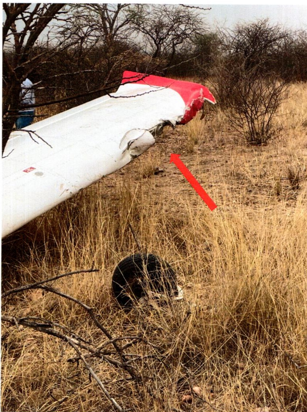
Image 5: Red arrow shows impact of bushes that struck left wing on landing.
