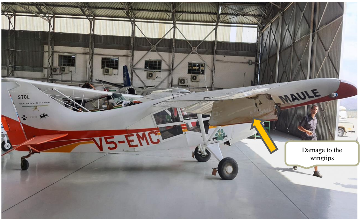
Figure 1: The damage at the wing tips...
