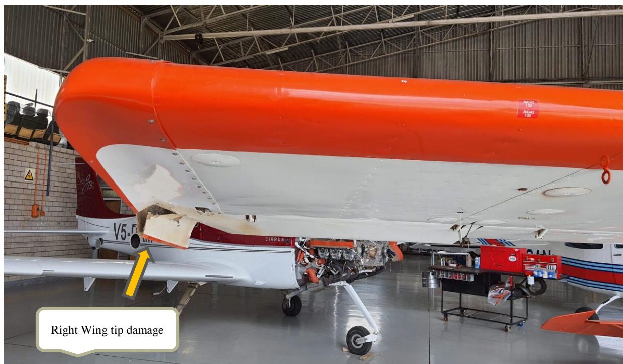
Figure 2: illustrating the carbon fibre wingtip, which was damaged.
