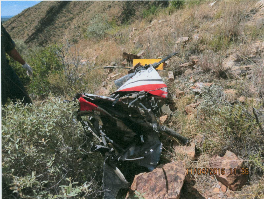
Image 8 - Rotor mast and gearbox found 117 meters from impact point
