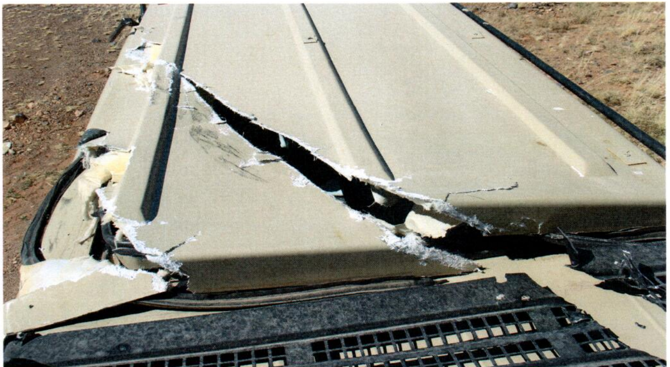
Figure 4: A picture showing the top of the vehicle that was damage by the two main rotor blades.
