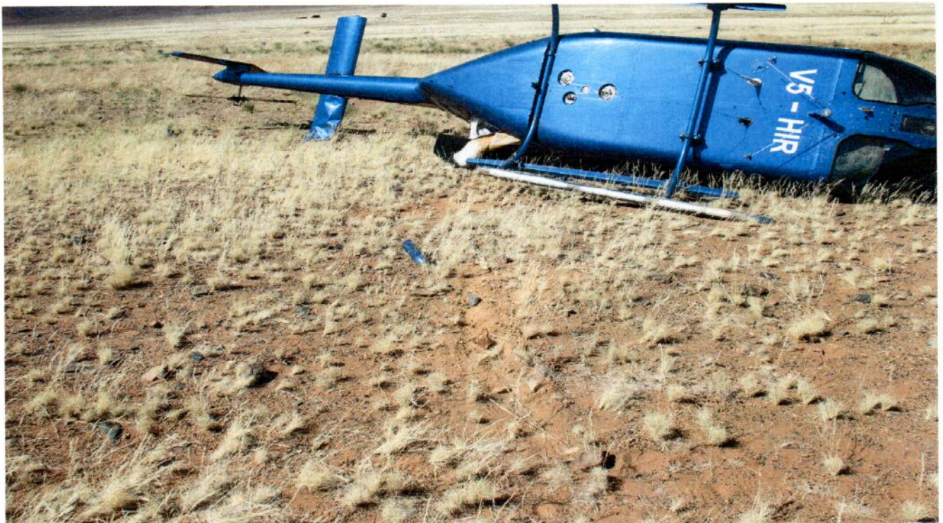
Figure 3: Picture showing a little damage to the belly and horizontal stabilizer
