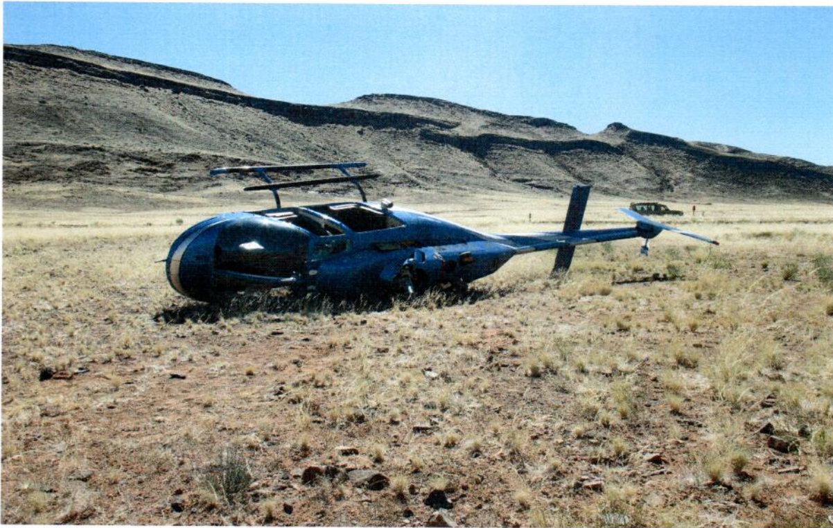
Figure 1: Picture showing damage to the aircraft especially to the main transmission system.
