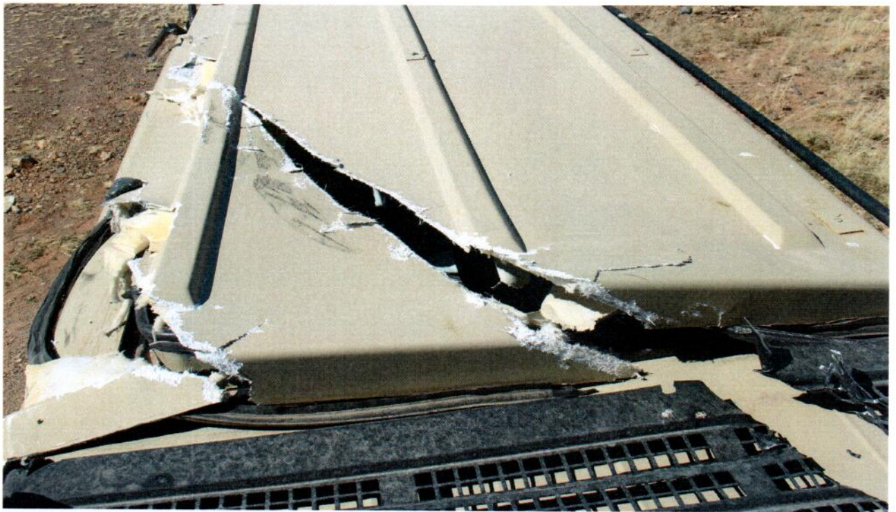
Figure 7: Picture showing the Vehicle top that was struck by the two main rotor blades
