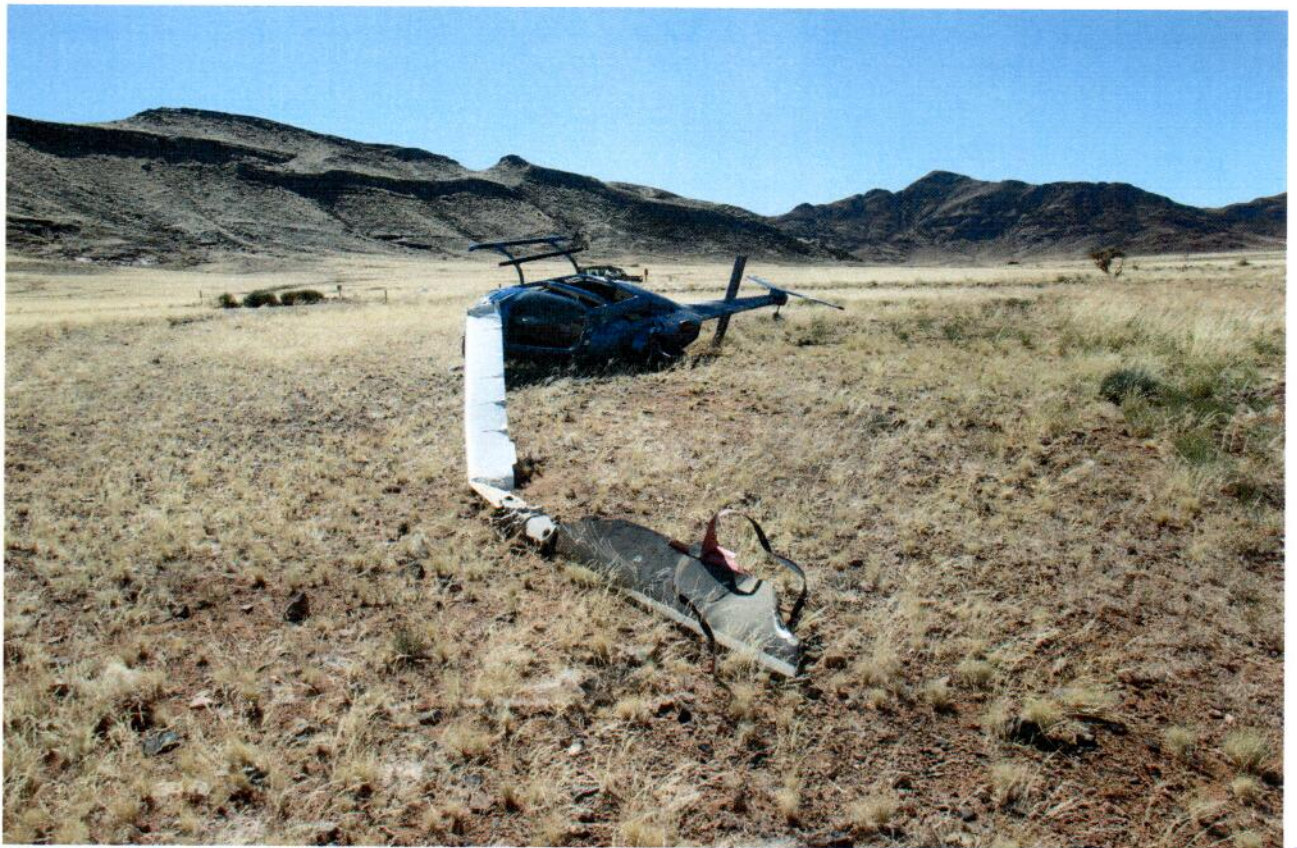
Figure 8: Picture showing the rotor head at 5 meters from the wreckage
