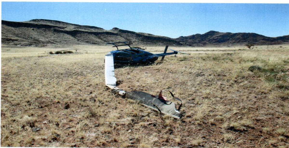
Figure 2: Picture showing the rotor head that broke off from the mast.
