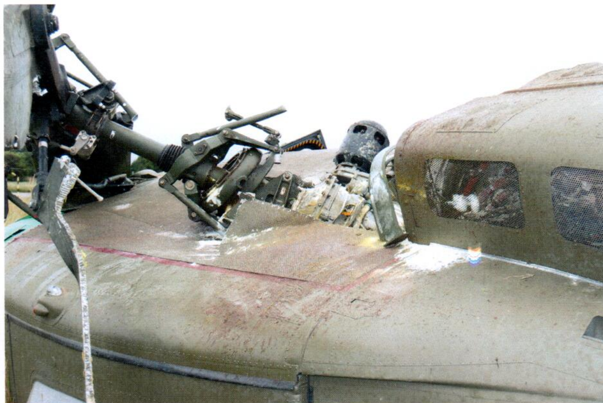
FIGURE 3: Photo showing the damage of the rotor blades, the broken transmission support platform and broken pitch change links.
