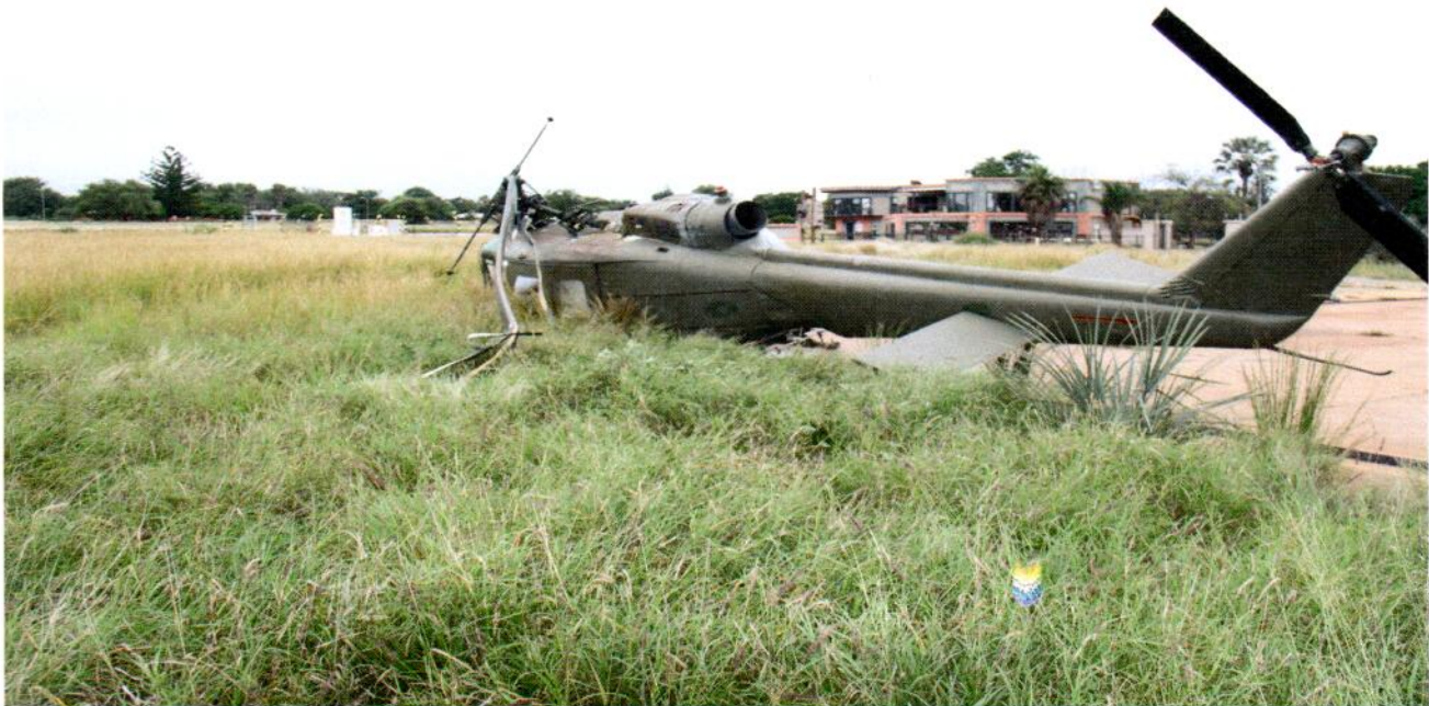
FIGURE 1: Photo showing the helicopter was substantial damage especially the transmission support platform.
