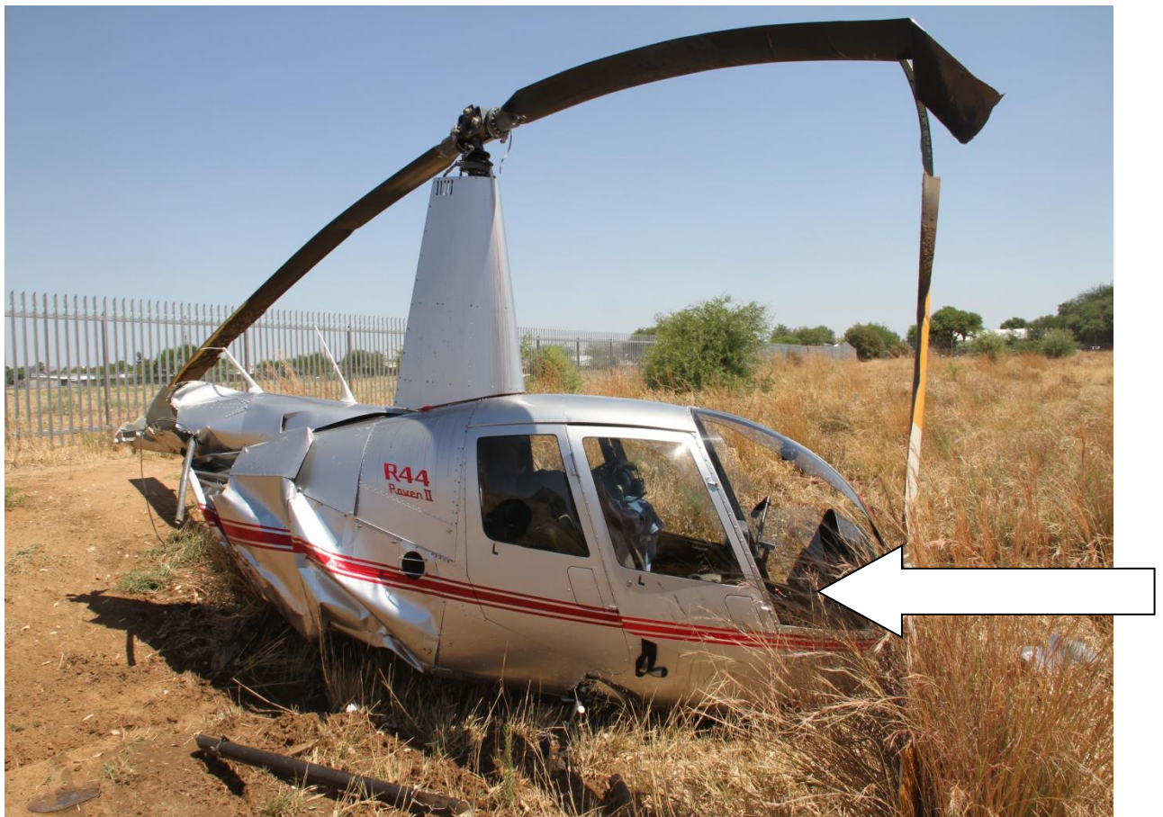
Figure 1. The photo indicating the wreckage of V5-HSF where it came to a halt after the accident. The arrow pointed at the shattered windscreen.
