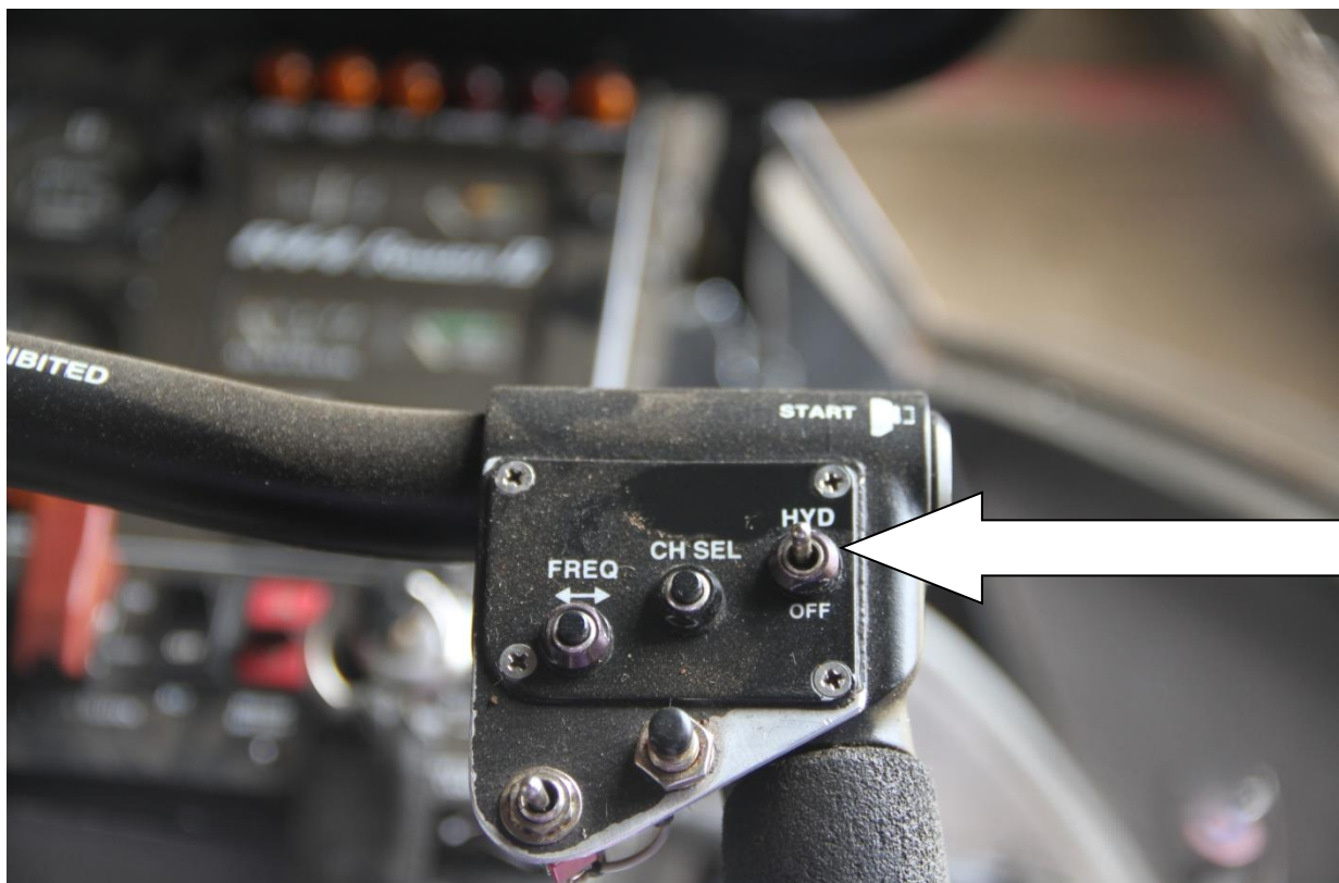
Figure 5. The photo indicating the position of the Hydraulic switch on the right end of the cyclic. The arrow indicating that the Hydraulic switch was switched "ON" during the accident.
