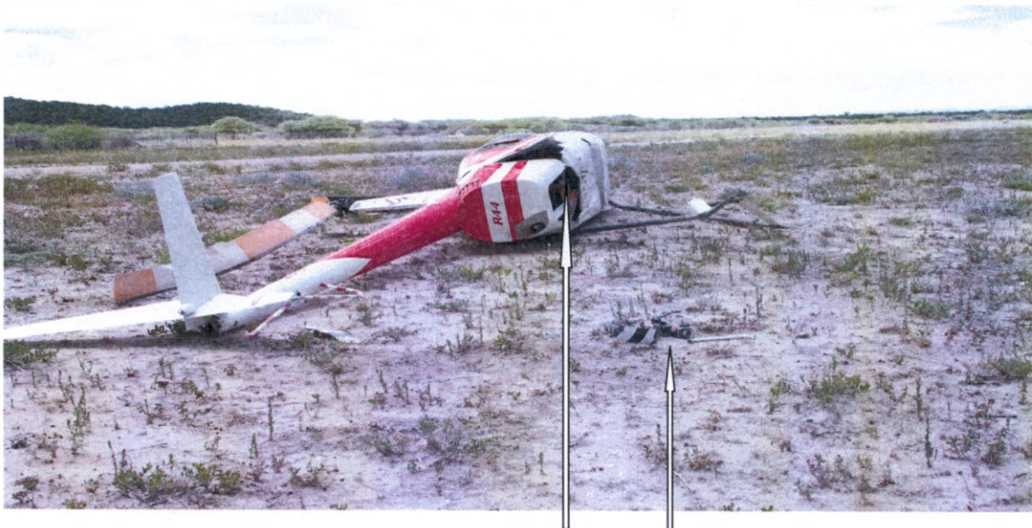
FIGURE 2: Photo showing the damage on the belly, broken off starboard skid and a detached tail rotor system.
