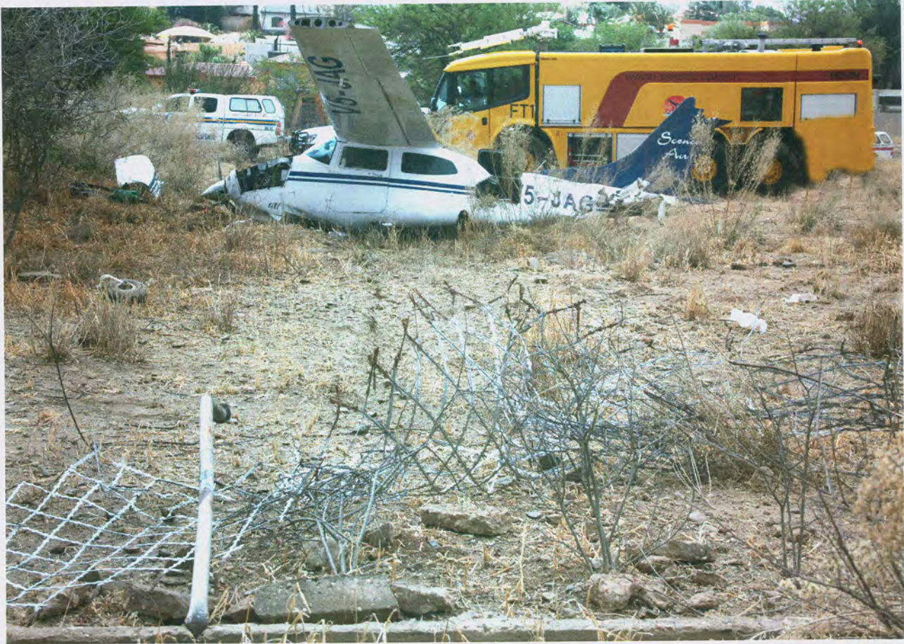
Figure 3: Damaged fence during impact sequence.
