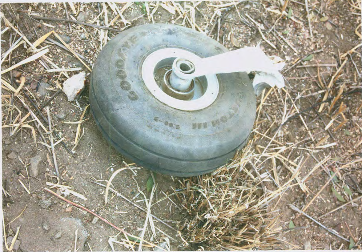
Figure 7: The nose wheel broken off due to high impact forces.
