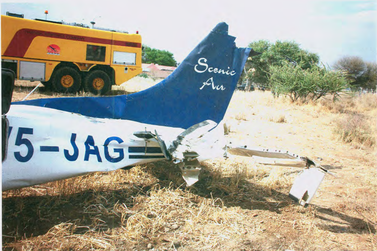
Figure 4: The damaged tail section.
