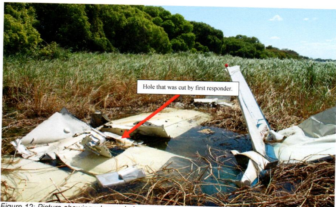
Figure 12: Picture showing where a hole was cut on top of the aircraft between the wings to gain access to the cabin.
