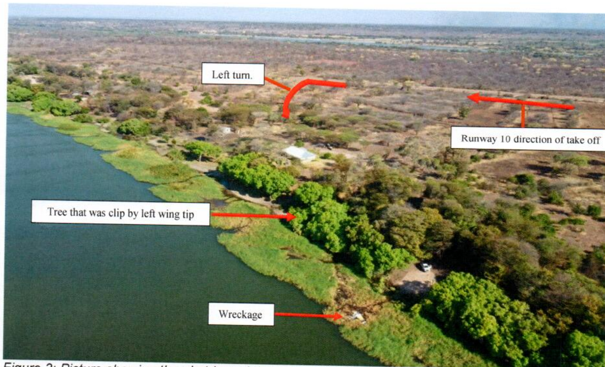
Figure 3: Picture showing the airstrip and the sequence of manoeuvres made by the aircraft.
