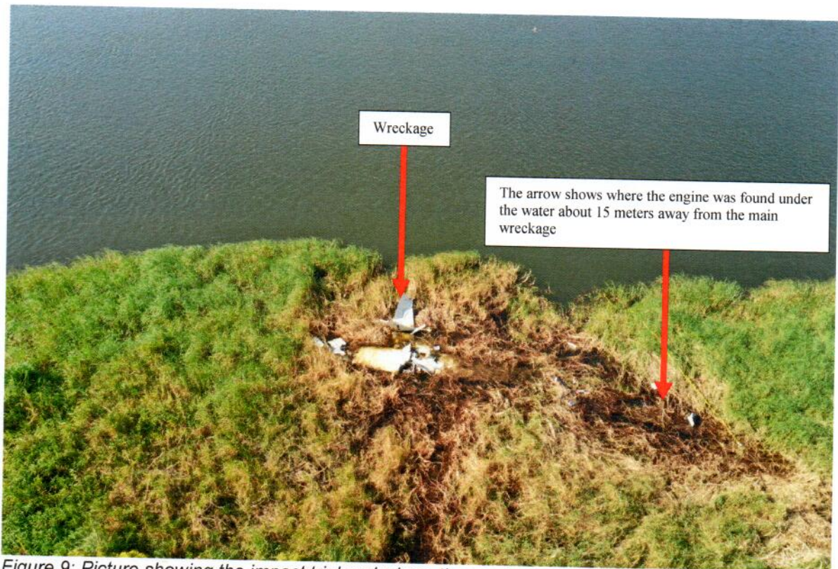
Figure 9: Picture showing the impact trail and where the engine was found (Drone image).
