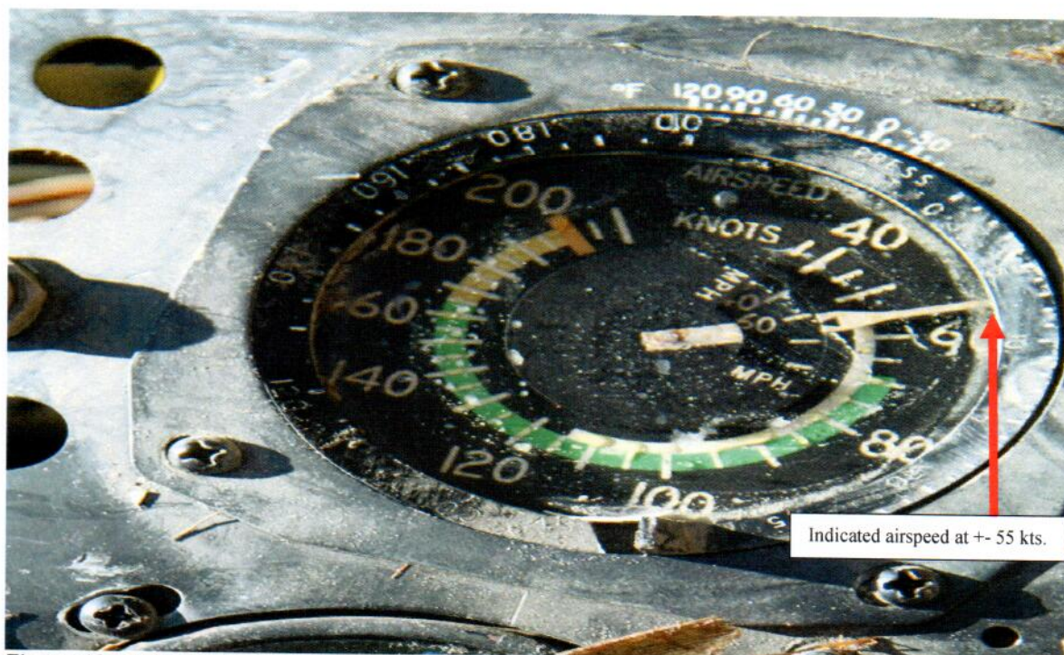
Figure 18: In the Picture the red arrow is pointing to the aircraft speed during the crash on the Airspeed indicator.
