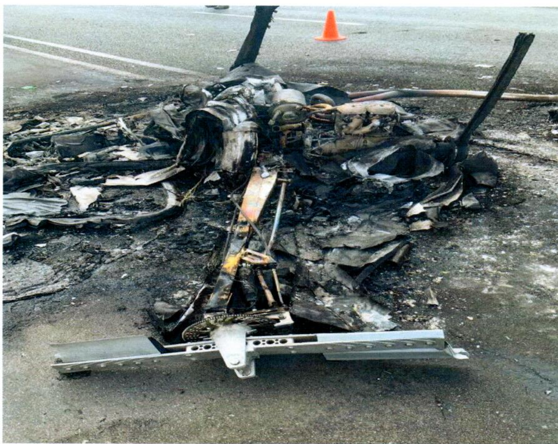
Figure 2: the wreckage laying across the road after hitting power lines.
