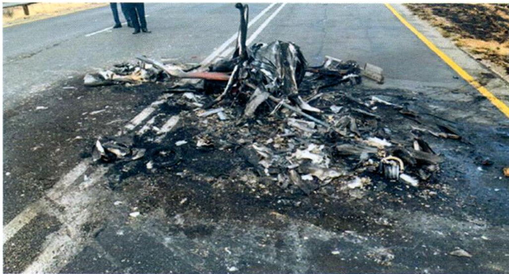
Figure 1: Gyrocopter destroyed then consumed by post impact fire.
