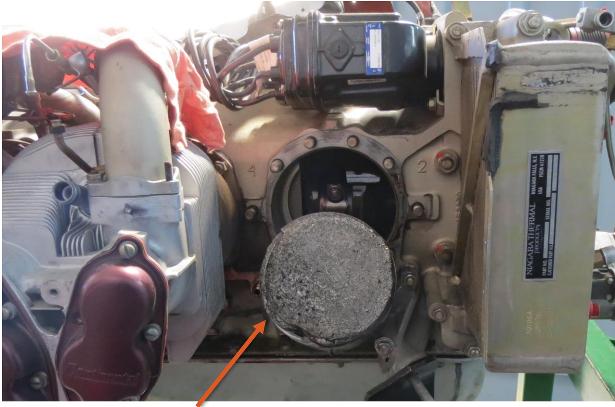
Figure 3. Piston no.2 exhibiting substantial wear.
