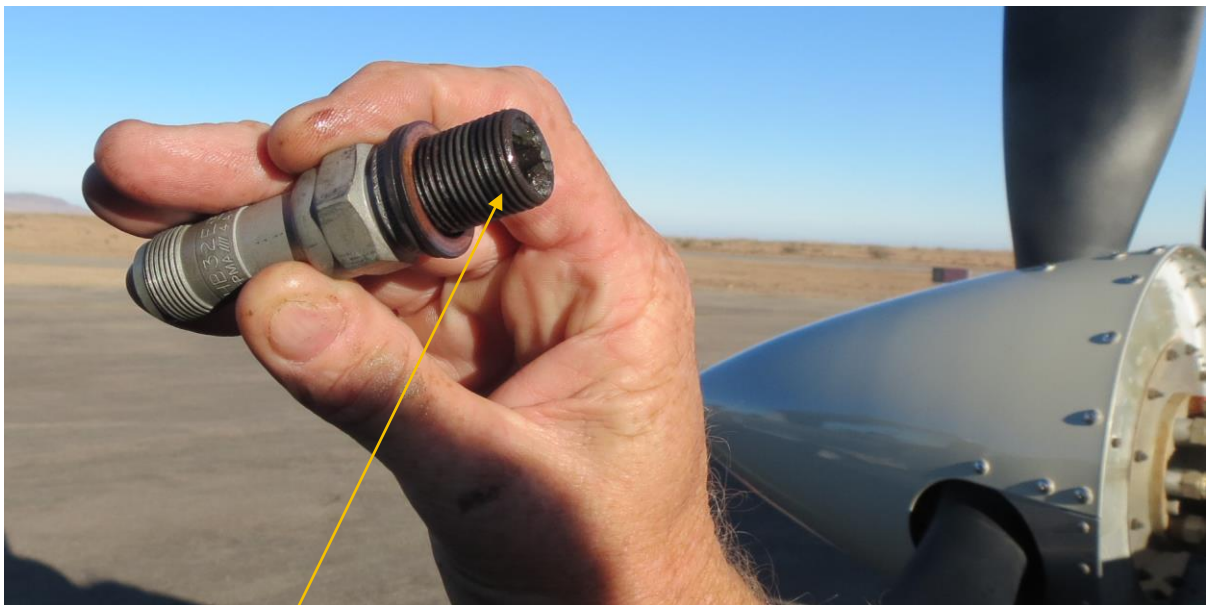
Figure 2. Metal deposits on the No.2 spark plug.
