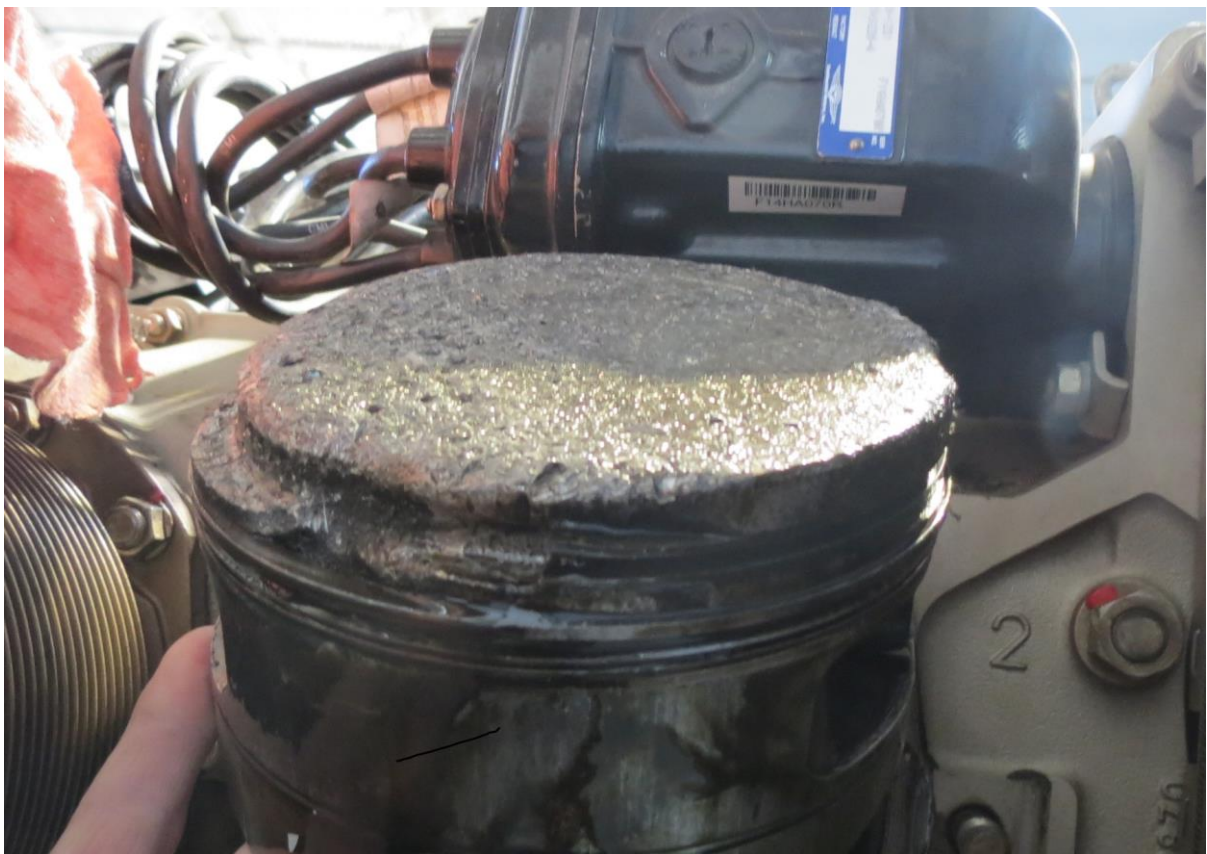
Figure 4. A close up view of the excessive heat damage on the piston head
