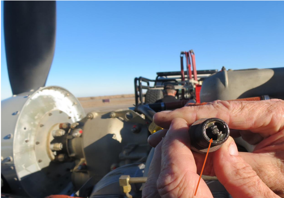
Figure 3. Grounded Spark Plug Electrodes on No.2 cylinder of the right engine.
