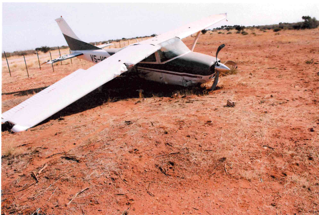
Figure 1: Damage to the lower fuselage, undercarriage, propeller and the wings.
