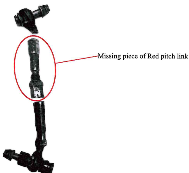
Figure 19: Picture shows how the missing piece of Red pitch link look like (Illustration).
