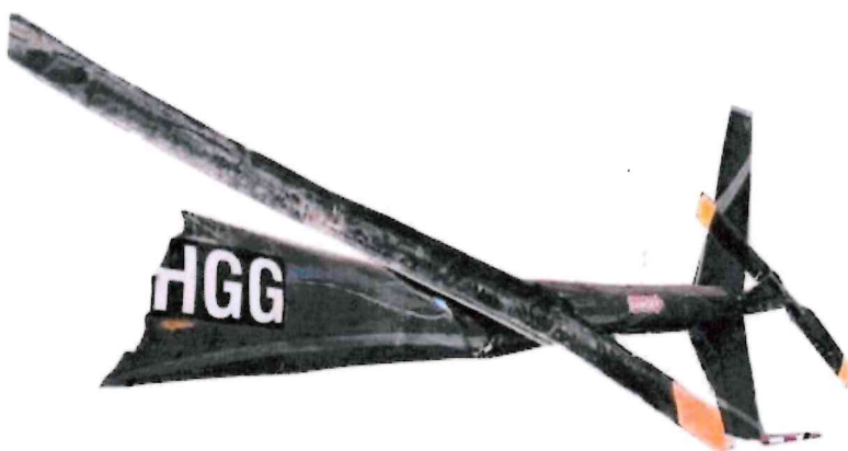
Figure 27: Image shows how the MR blade made contact with tailboom (Illustration).
