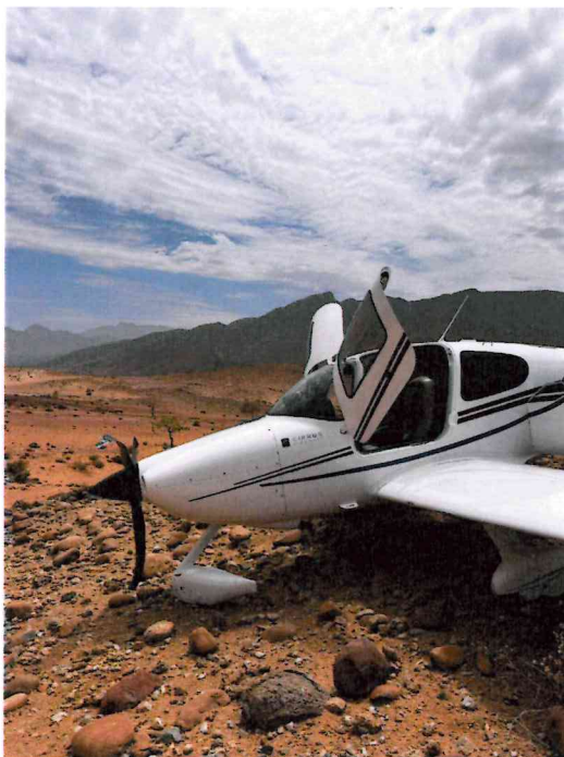
Figure 2 and 3: Pictures shows how the propeller was damaged.
