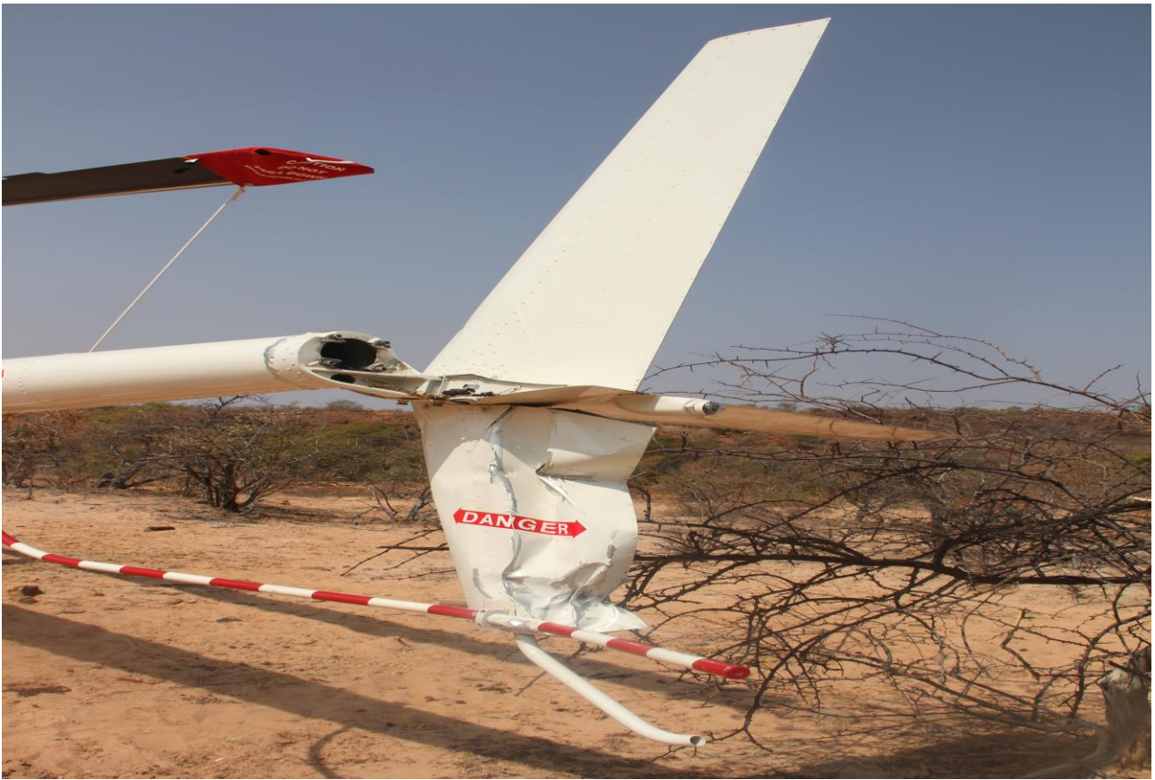
Figure 3. Closer view of the aft tail boom structure with the tail rotor assembly absent.
