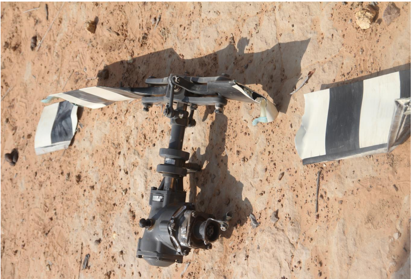
Figure 4. The tail rotor assembly that broke off with both rotor blades being fractured.
