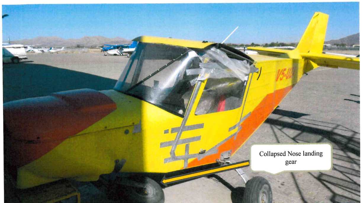
Figure 2: Photo depicting the aircraft's nose wheel strut collapsed...
