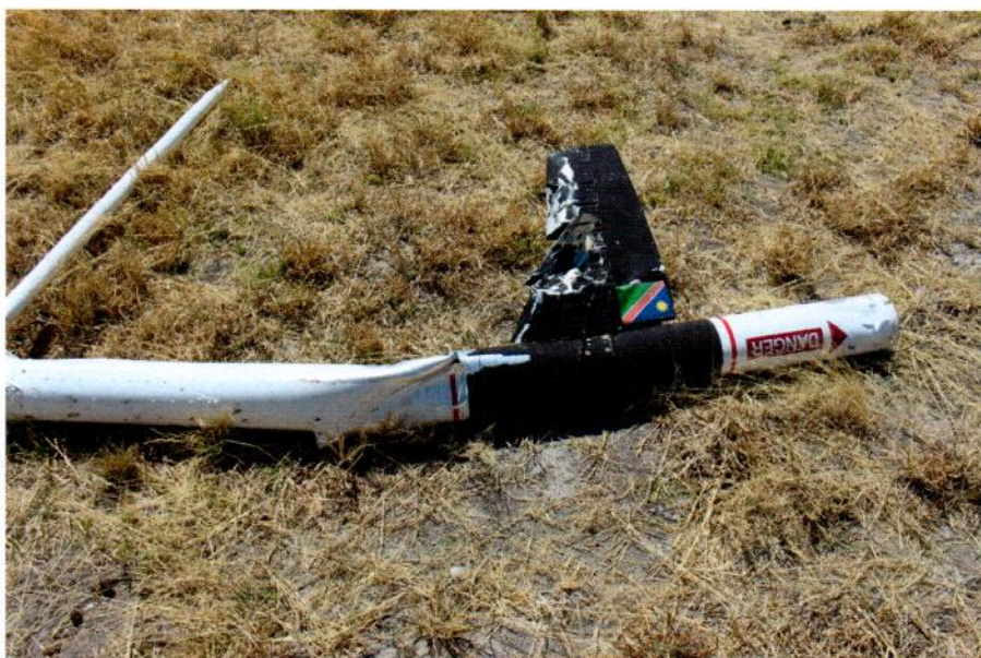
Image 5 Tail boom was struck and destroyed by the main rotor blades during excessive flare in landing phase.
