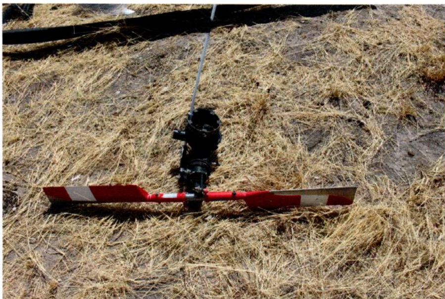
Image 4 Tail rotor blades shows low rotational speed impact damage.
