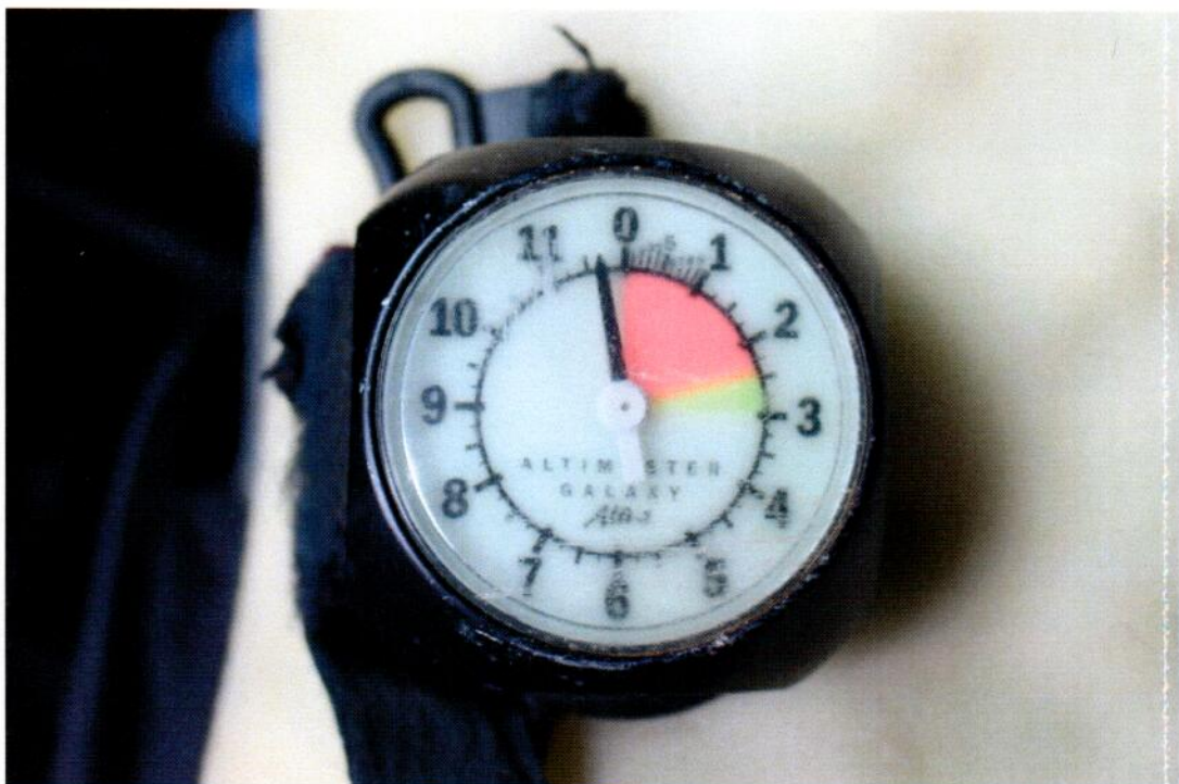
Image 6: Altitude meter clearly indicating the caution (yellow) and danger zone (red) for deployment
