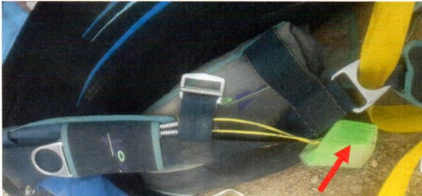
Image 1: Unsuccessful reserve chute deployment handle (red arrow)
