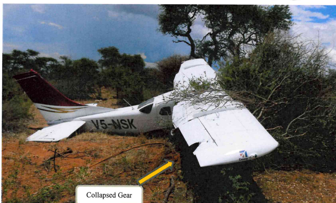
Figure 1: Collapsed landing gear.
