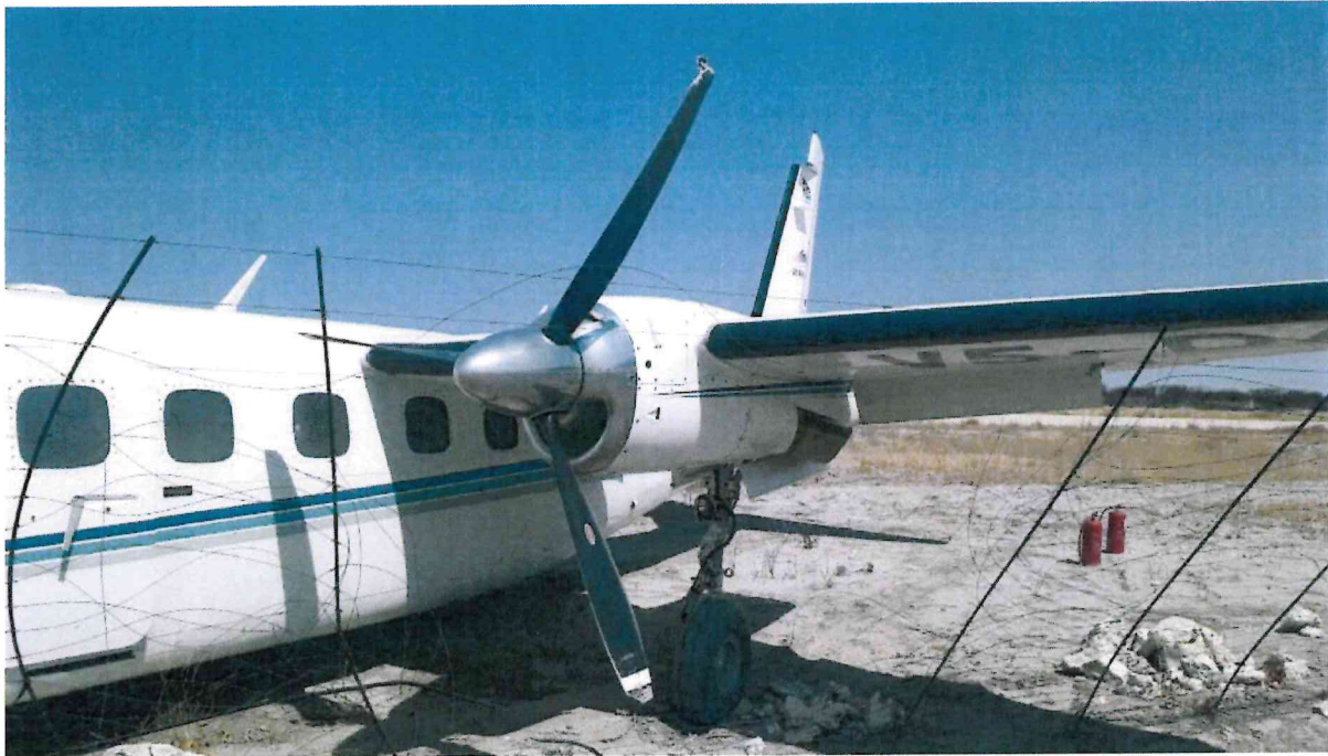
Figure 3: Picture showing the damage to the left propeller.
