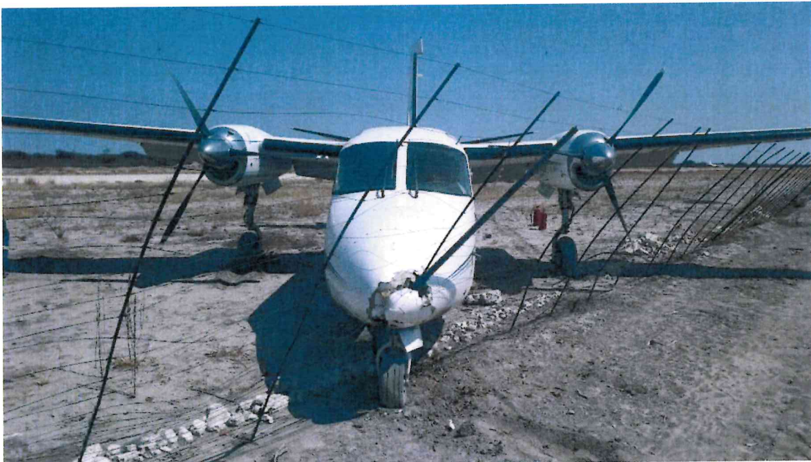
Figure 3: Picture showing the damage to the nosecone.
