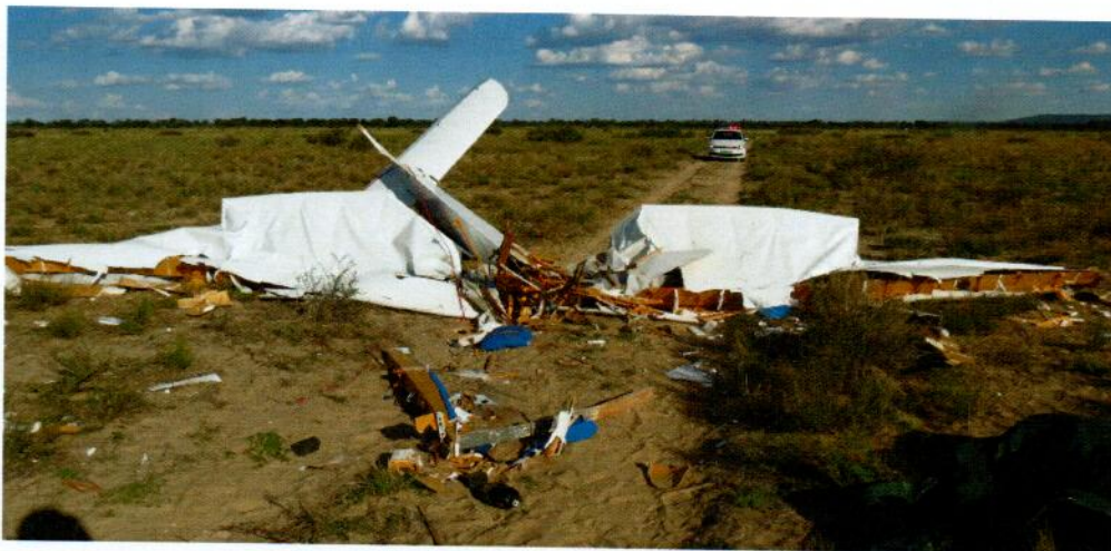
Figure 1: Extent of damage on the fuselage and relatively small radius of wreckage distribution.
