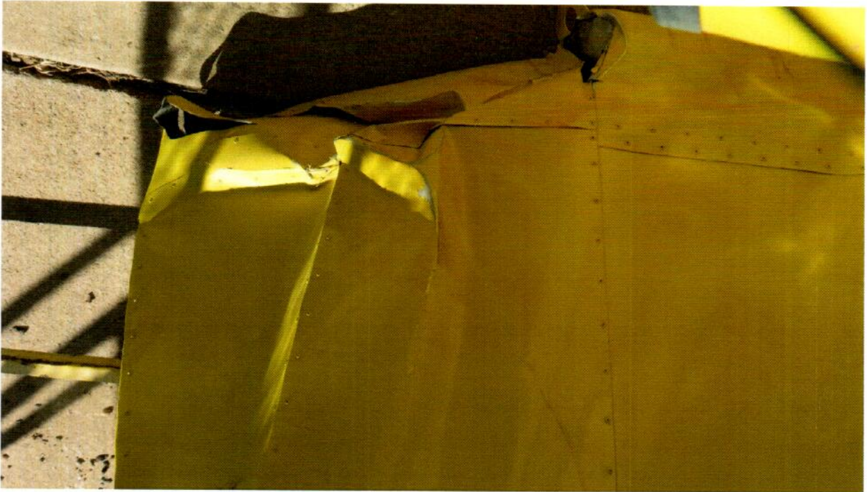
Photo 5. Photo depicting the aircraft's left wing tip after hitting the bushes
