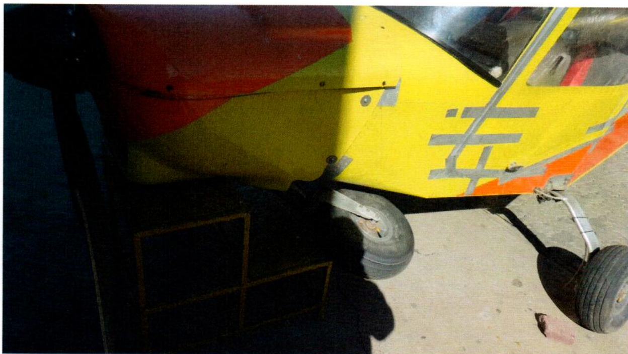
Photo 4. Photo depicting the aircraft's Nose wheel strut collapsed..
