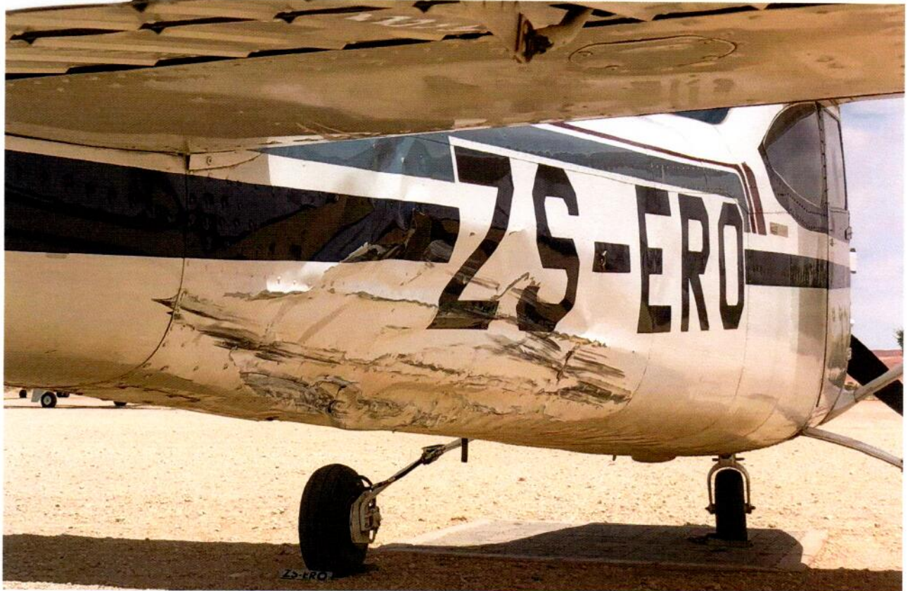
Photo 1. Damage to aircraft's rear fuselage.
