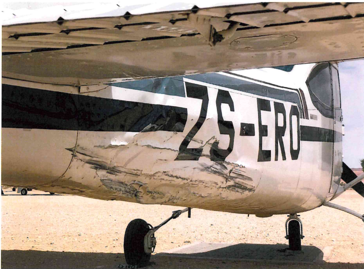
Figure 1. Damage to the lower aft fuselage appr. 1,5 m behind the right door.
