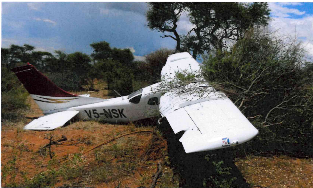
Figure 1. Photo of damaged aircraft as it hit the bush
