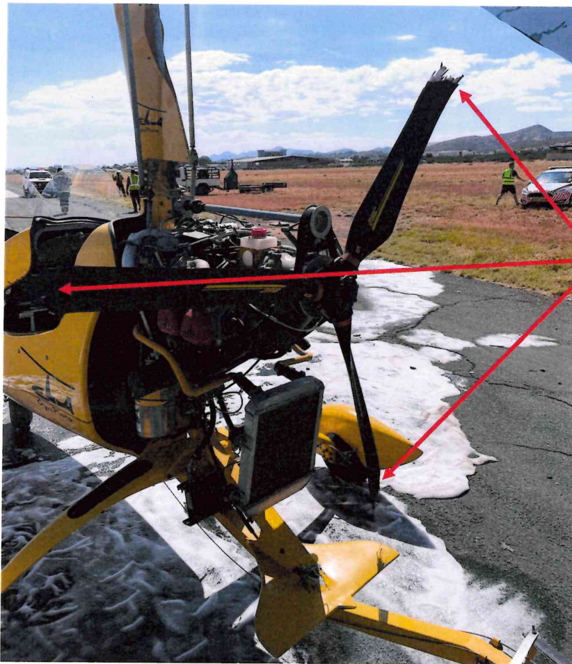
Figure 6: Photo depicting damage to the engine propeller.
