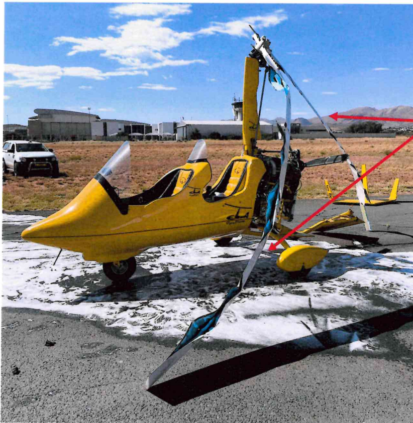
Figure 5: Photo depicting damage to main rotor.
