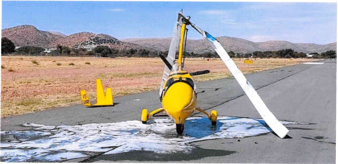
Figure 4: Photo depicting overall damage to Gyroplane.
