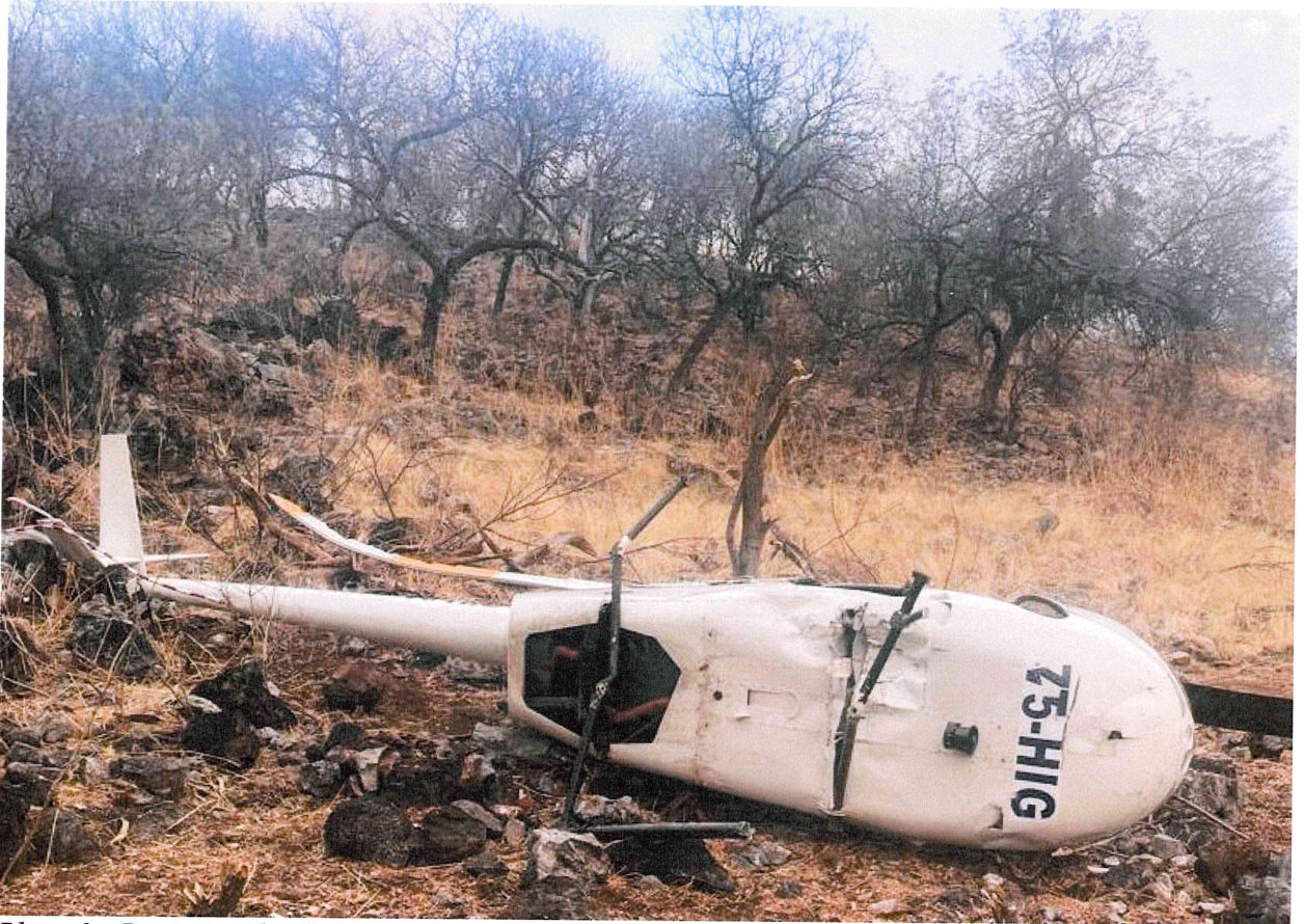
Photo 2 : Depicting the damage to the under carriage
