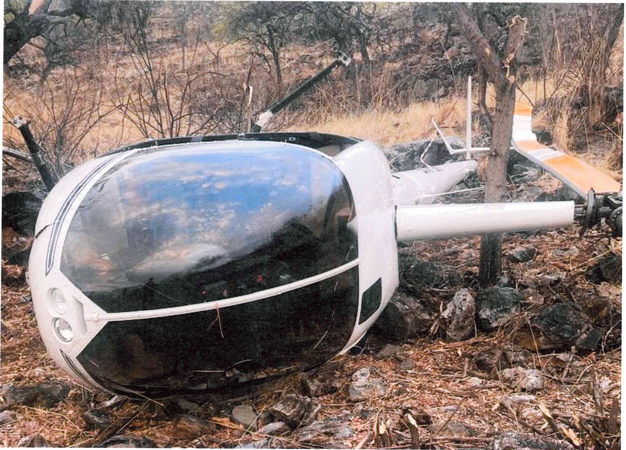
Photo 1. The helicopter rolled onto its left side after impacting the trees.
