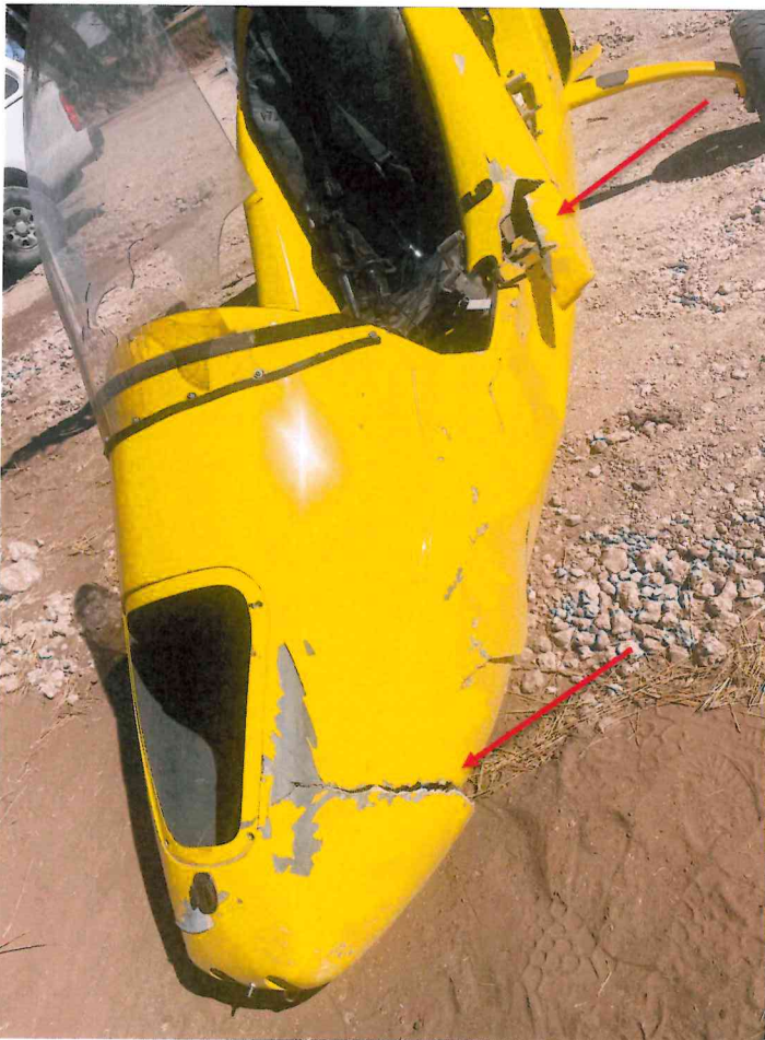
Figure 6: Picture showing the damage to the fuselage (Red Arrows)
