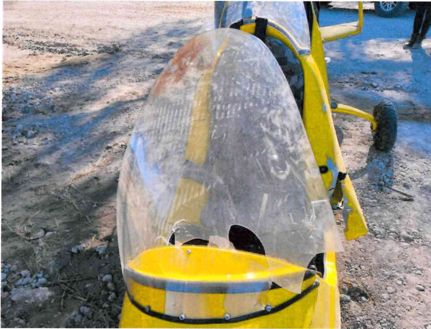
Figure 7: Picture showing the damage to the windshield.
