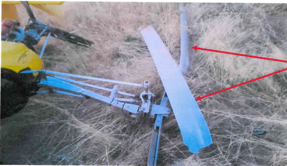
Figure 5: Picture showing the damage to the main rotor. (Source: Namibian Police)
