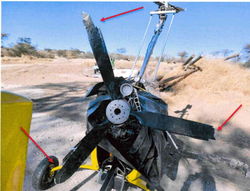
Figure 8: Picture showing the damage to the pusher propeller at the back of the engine (Red Arrows).
