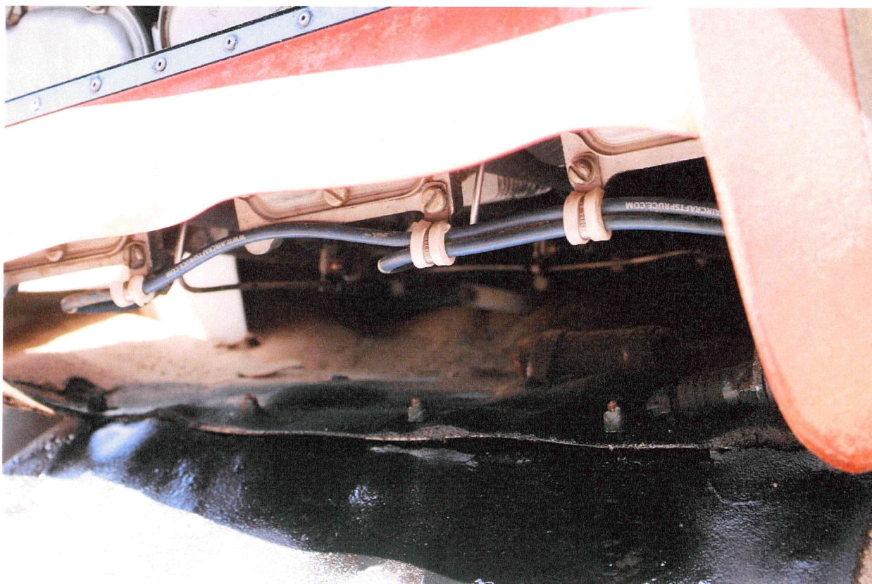
Photo 3: Loss of engine oil.
