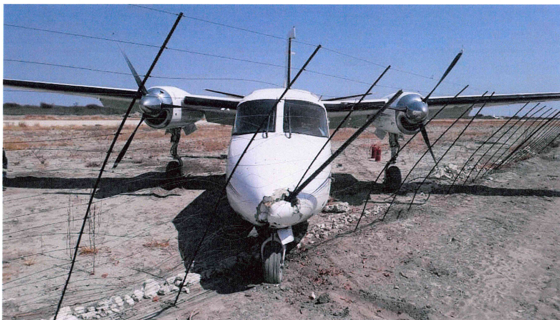
Figure 3: Picture showing the damage to the nosecone.
